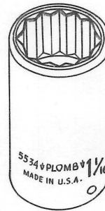
WRENCH-SOCKET, ENGINE MOUNT ATTACHING BOLT 1/16 INCH OPENING
